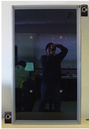
Figure 4. ECS Display with diagonal camera arrangement and LED markers in visible light.
