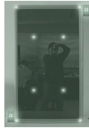
Figure 5. ECS Display with diagonal camera arrangement and LED markers in infrared light. Note the illumination of the LED markers on the screen.
