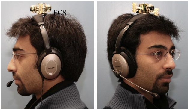
Figure 1. Attentive Headphones with embedded eye contact sensors (front and back) and microphone.
